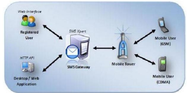
Gambar 5 Skema SMS Gateway
